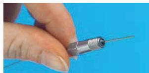
The ferrule will be properly seated, and should remain in place when light force is applied. If it slides loosely on the column, repeat procedure.
