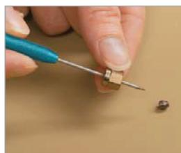
Dislodge a stuck ferrule quickly and easily—without scoring the fitting.
