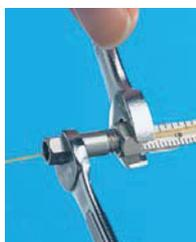
Tighten the assembly to ensure a properly seated ferrule. Loosen the assembly and remove the column and column nut.
