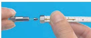
Install the column nut and ferrule onto the column. Slide the column into the installation gauge to the recommended insertion distance. Finger-tighten the nut.
